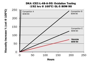
In the DKA oxidation test, product performance is measured by how much harmful viscosity increase will occur over time (therefore, the flatter the line the better). Compared to these competitors, Petro-Canada's TRAXON with its advanced formulation is clearly superior.
